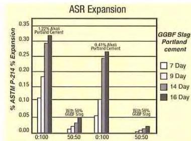
ASR Expansion. Reduced alkali-silica reaction
