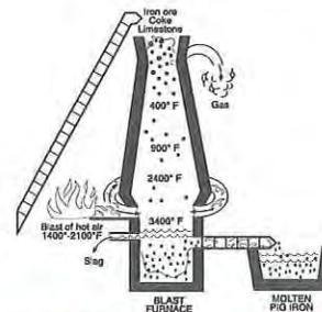
Iron and slag making process through a blast furnace.
