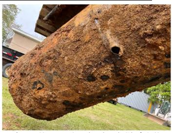
Photo No. 20 Apparent Geoprobe Hole on the Side of UST-03
