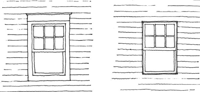
The loss of trim around windows is one of the most significant impacts of an over-siding job. The window shown here on the left has its original trim. Though rather plain, it gives character to the window. The trim around the window on the right was covered or removed, lessening the character of the window.
