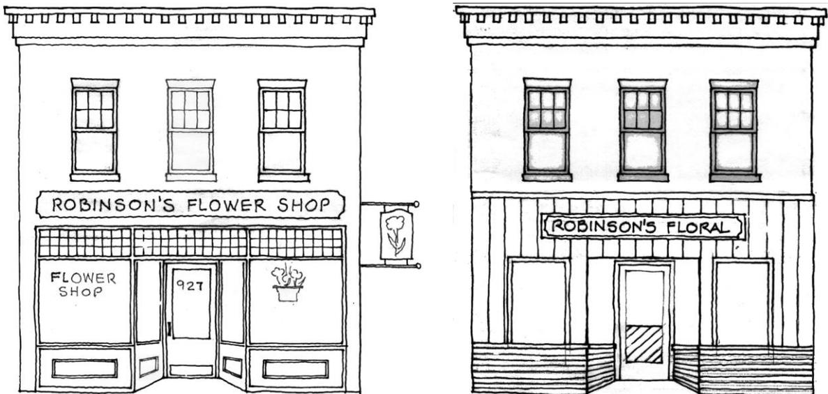
Appropriate sun control devices on traditional storefronts include awnings, blinds, curtains, and clear ultraviolet films. If security grilles are essential, mounting them inside the glass, rather than outside, is preferred. Accordion or scissor gates are not appropriate.
