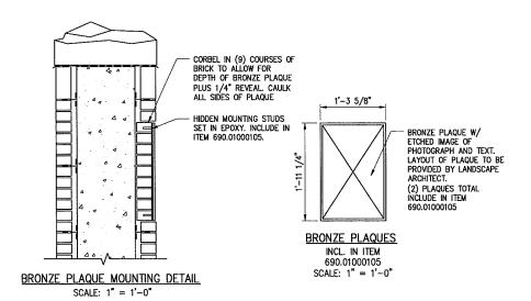
NOTE: CONTRACTOR'S OPTION TO COORDINATE PLAQUE DELIVERY WITH CONCRETE SIDEWALK POUR TO SET PLAQUES WITH -FORM OPENING TO RECEIVE BRONZE MOUNTING STUDS IN WET CONCRETE. PLAQUES 1/8" LARGER THAI PLAQUE ON ALL -CONCRETE SIDEWALK ITEM 608.0101 -- DRILL INTO CONCRETE AND EPOXY SIGN STUDS INTO
