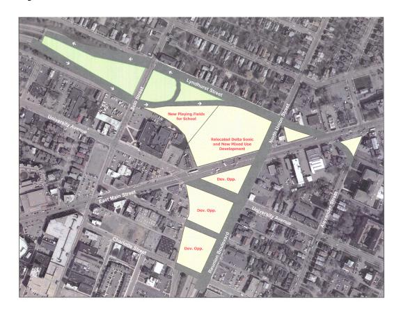
**University Avenue Inner Loop Interchange Concept** – This option provides a direct connection to the Inner Loop from University Avenue by providing separate ramps to East Main Street (existing) and the new ramps to University Avenue. This option has the following to offer:
