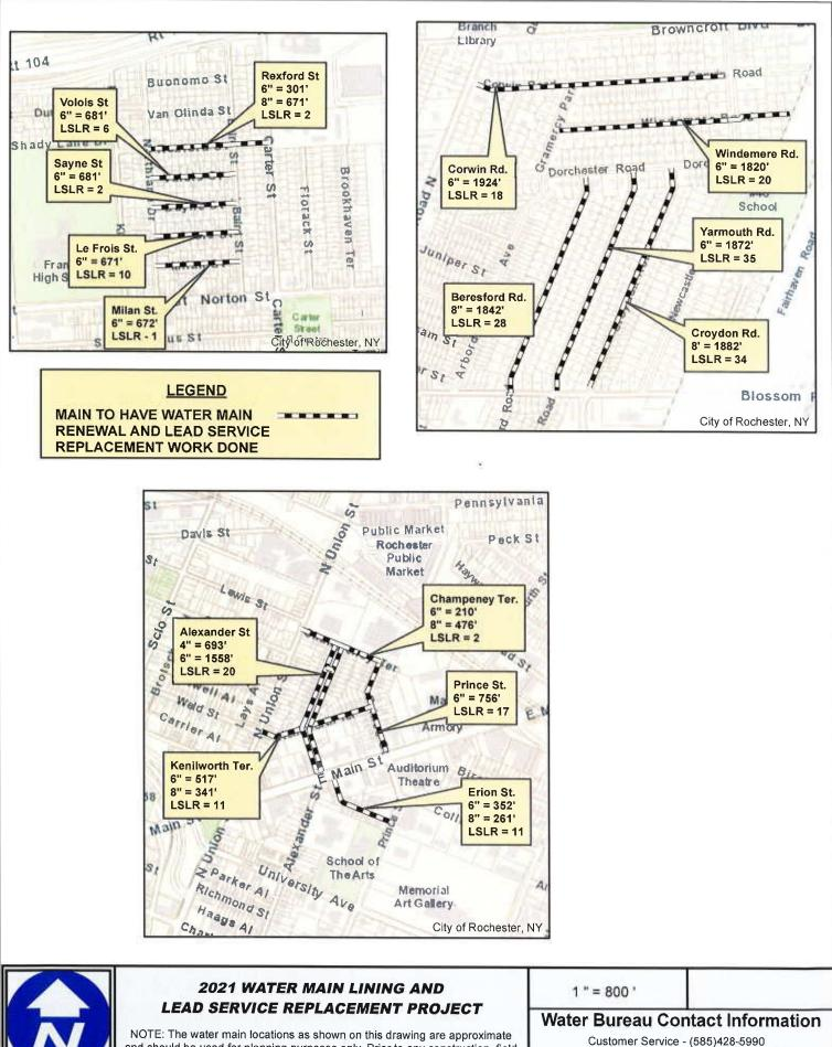
and should be used for planning purposes only, Prior to any construction, field locations should be verified by calling Dig Safely New York at 1-800-962-7962. Customer Service - (585)428-5990 Water Bureau Dispatch Office - (585)428-7500 Water Bureau Maps & Records - (585)428-7562
