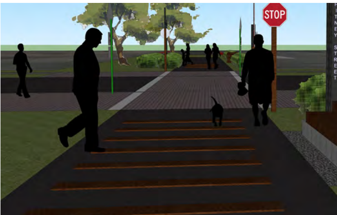
Embedded Railroad Ties - Railroad ties embedded in the pavement can not only interpret the railroad history of the corridor but also act as a tactile warning strip for trail users approaching a road intersection with the TrailRoad.
