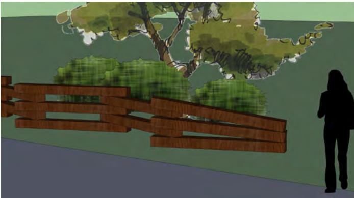
Zig Zag Fence Concept - A zig zag fence made up railroad ties can be used to delineate trail edges and act as a safety barrier between incompatible uses and steep embankments.
