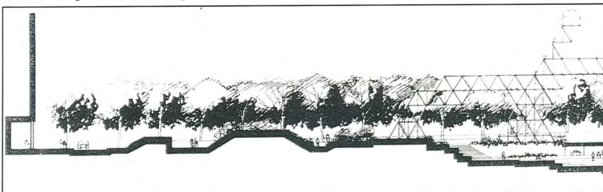
Section through South Berm illustrating visual and physical barriers
