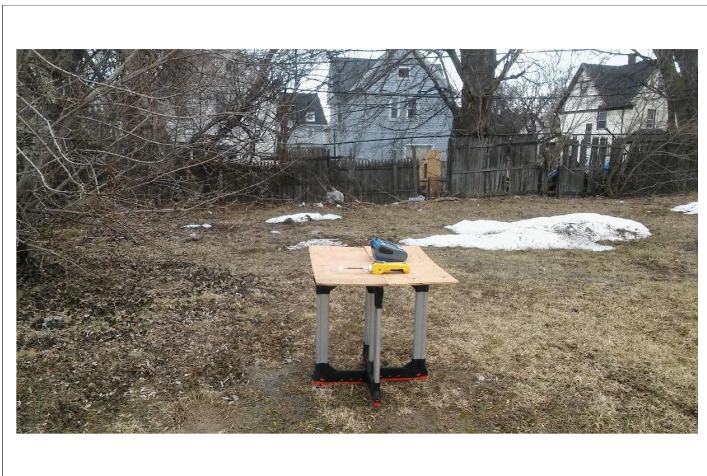
Air Monitoring Station with Dust Trac and PID meters
