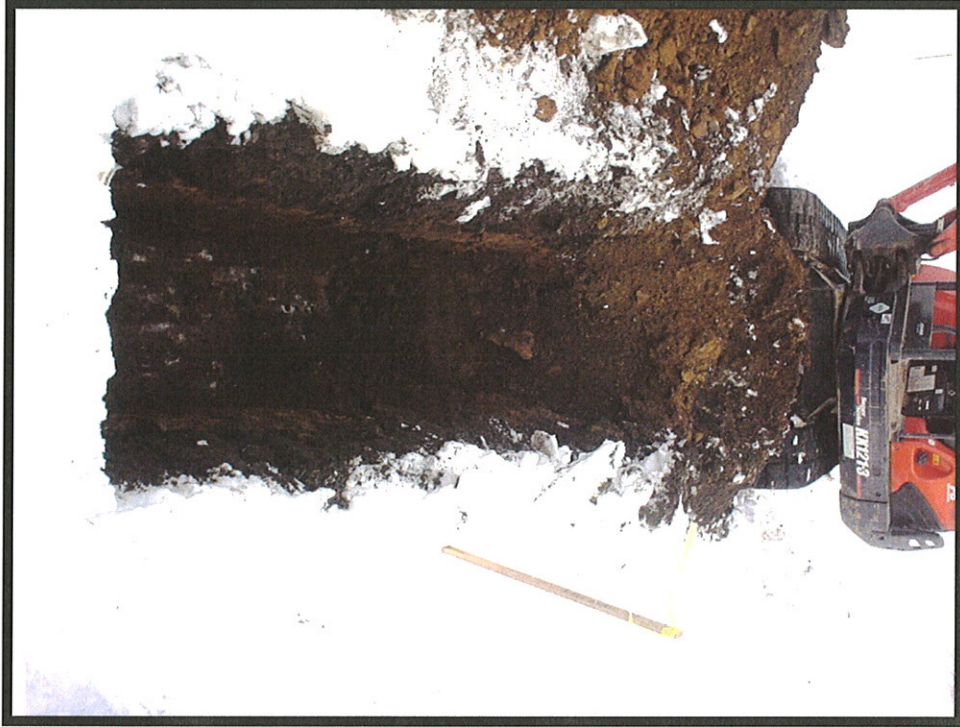
View of the TP-112 showing top of bedrock
