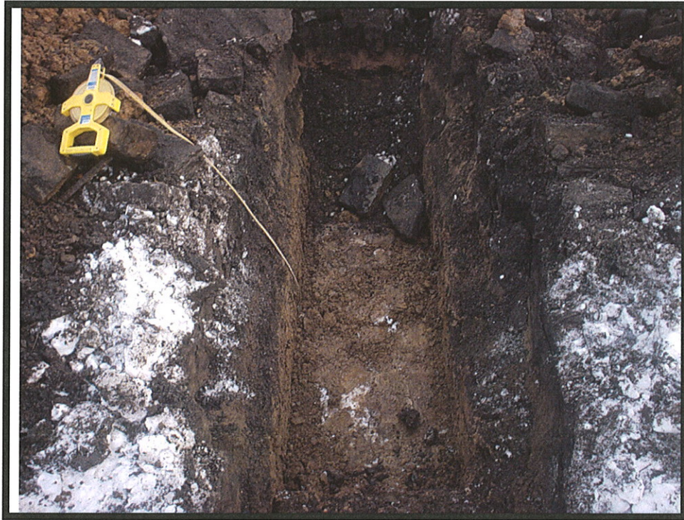
View of the TP-102 showing top of bedrock
