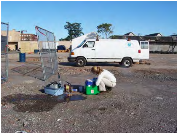
Photo No. 45 – Low-flow groundwater sampling at MW-06, 2008.
