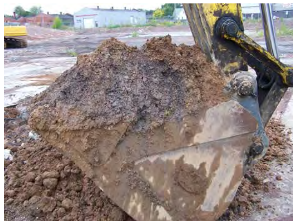
Photo No. 42 - Grey petroleum-discolored soil from 9 to 11 ft. bgs in TP-03, 2008.
