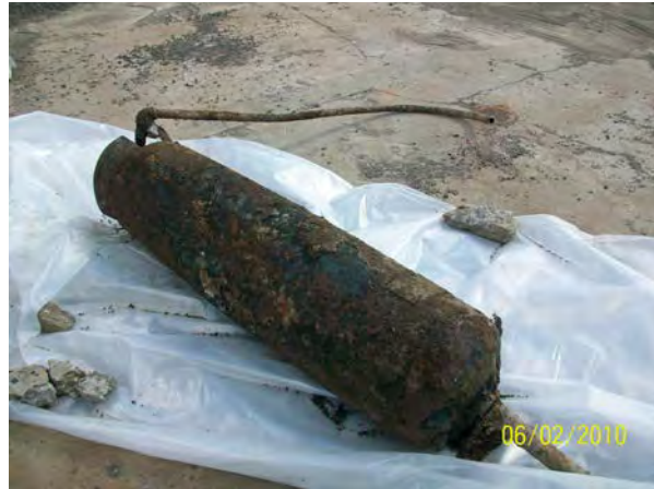
Photo No. 56 – AOC-3: Empty hydraulic oil tank from vehicle lift.
