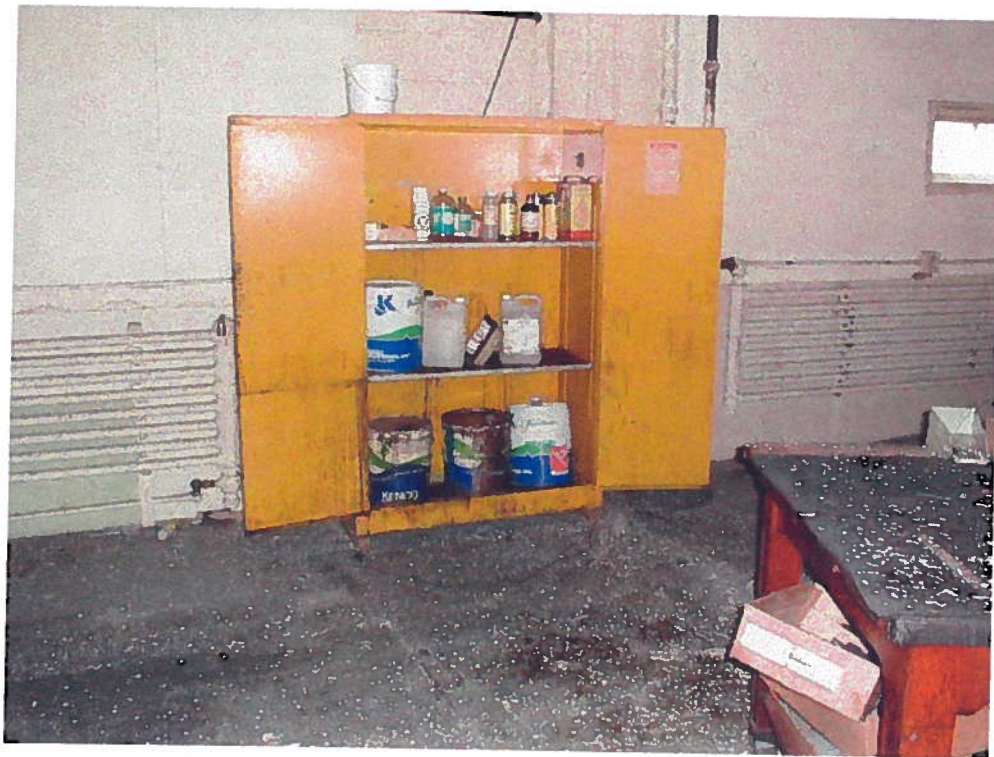
367 Orchard Street; flammable liquids, staining on bottom shelf; 3 rd floor
