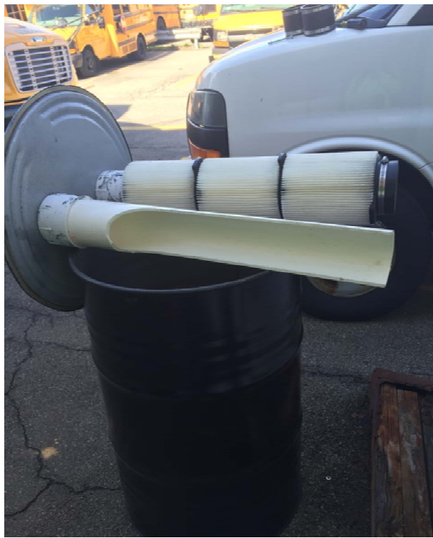
Knock-out tank filter (April 2017)
