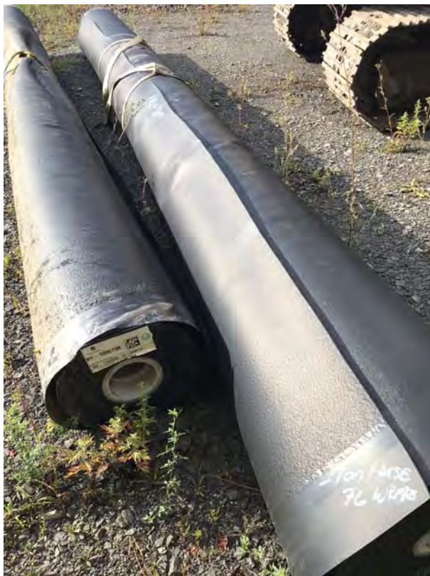
60-mil liner used for staging areas and decontamination pad (9-4-2019)
