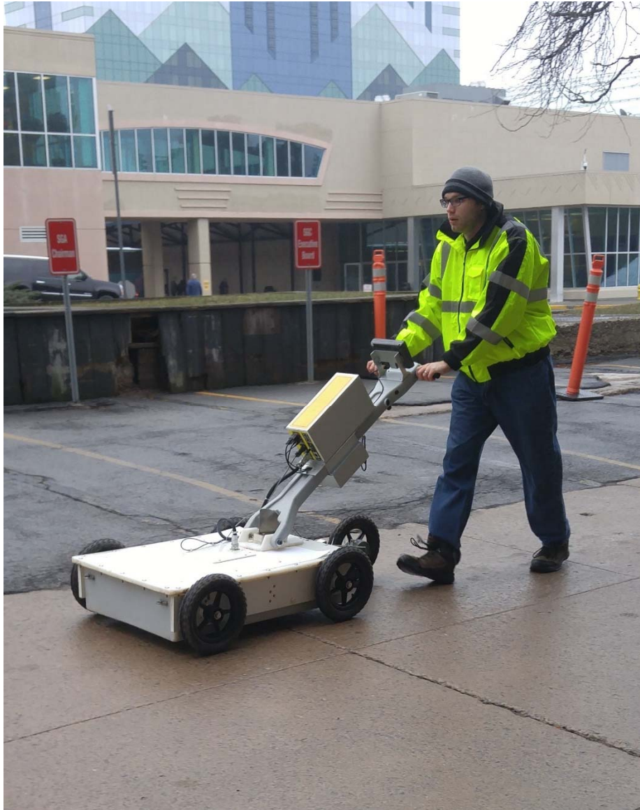
Figure (1). 300MHz IRIS GPR used for State Street Inspection
