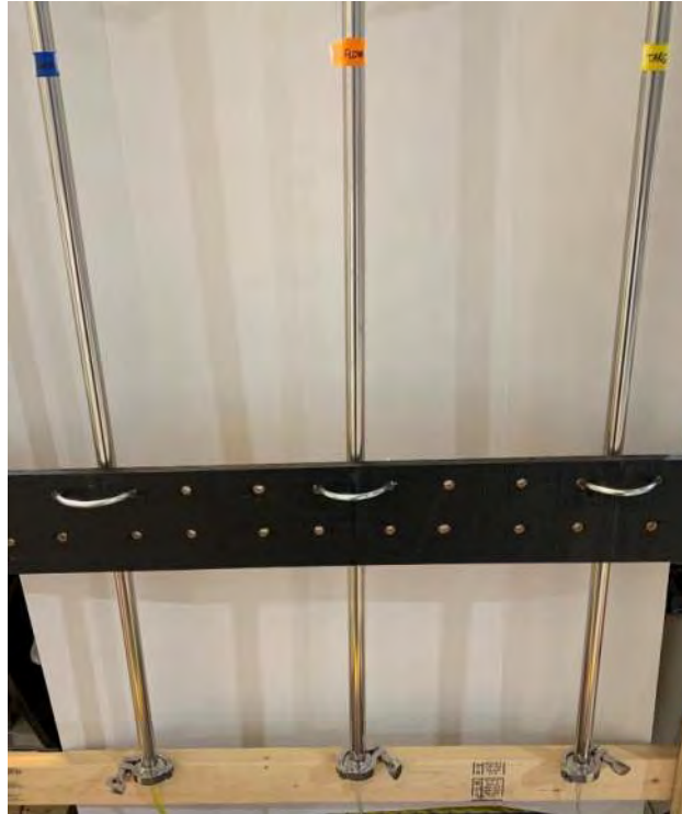
Photo 3. ZVI Column Test – 4-foot columns from left to right: Control, 5% Ferox Flow, 5% Ferox Target
