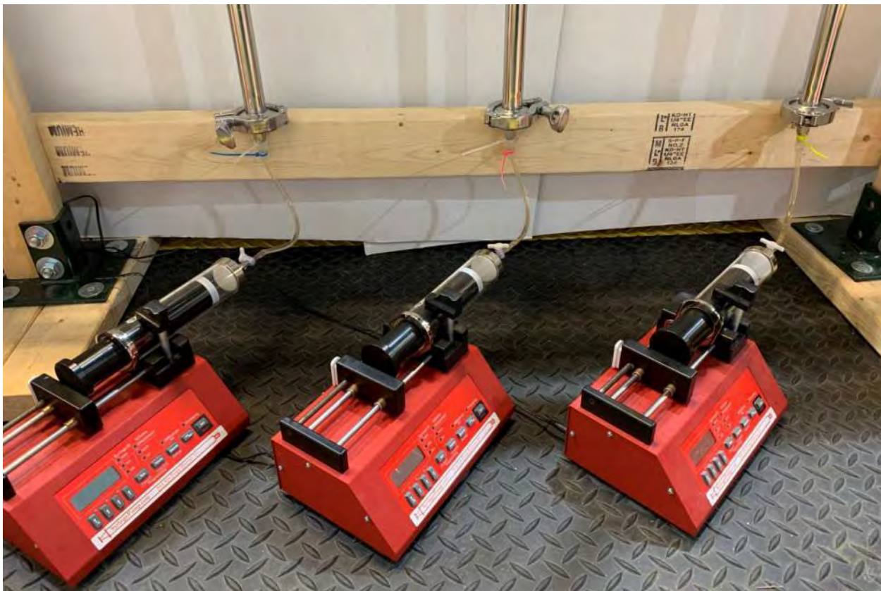
Photo 2. ZVI Column Test – Syringes, syringe pumps, column inlets
