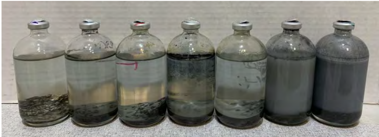
Photo 1. ZVI Kinetics Batch Test – from left to right: Control, 1% Ferox Flow, 5% Ferox Flow, 1% Ferox Target, 5% Ferox Target, 1% eZVI, 5% eZVI
