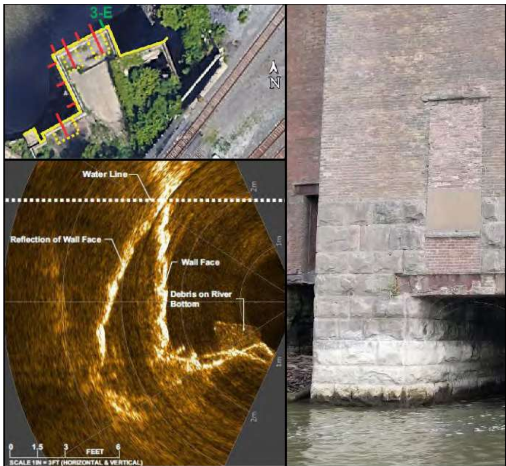
Figure 5 - Sonar Profile of Foundation
