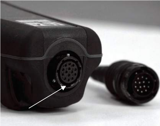
Figure 4, Note the keyed connector.
