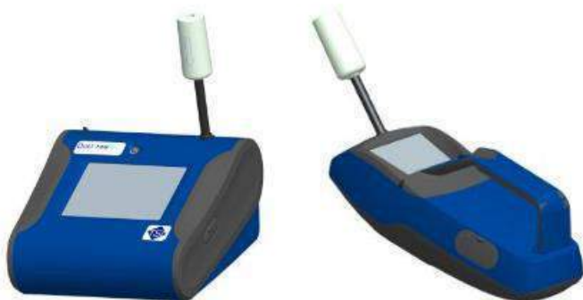
Figure 4-1: Attach Zero Filter to Inlet
