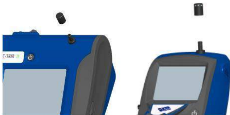
Figure 2-6: Putting on Inlet Cap
