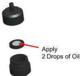
Figure 4-4: Apply 2 Drops of Oil to Impactor Plate
