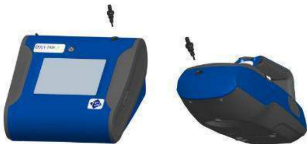
Figure 4-2: Unscrew Inlet Nozzle
