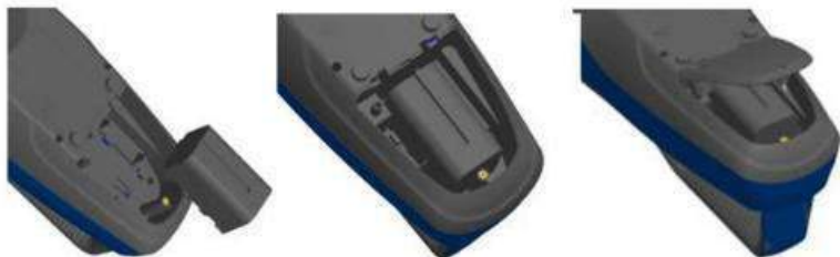
Figure 2-2: Batteries into Handheld Unit
