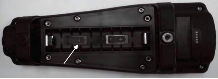
Figure 1, Pro20 with battery cover removed. Note battery symbols indicating polarities.
