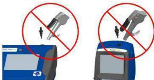
Figure 4-3: Do NOT Blow into Instrument
