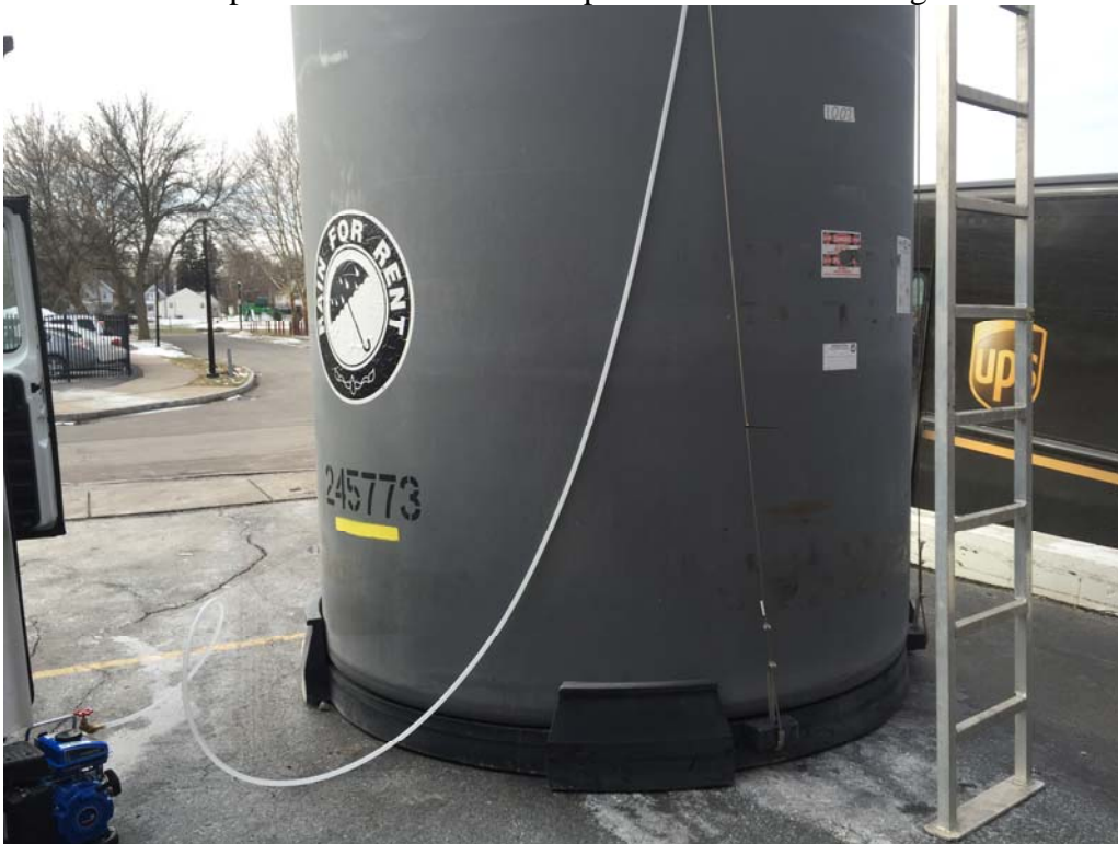
Frac tank that was located on south portion of Site for storage of development water from bedrock monitoring wells
