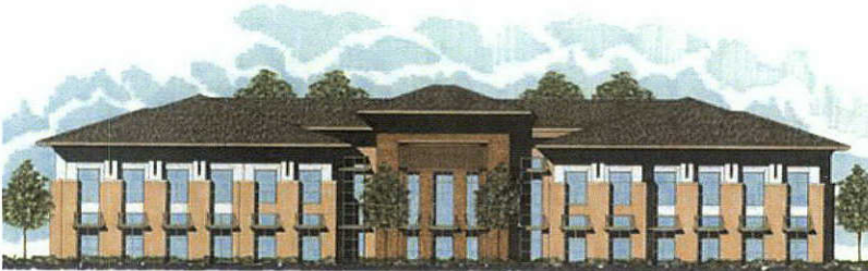
FIGURE 6 Recessed entry provides visual articulation
