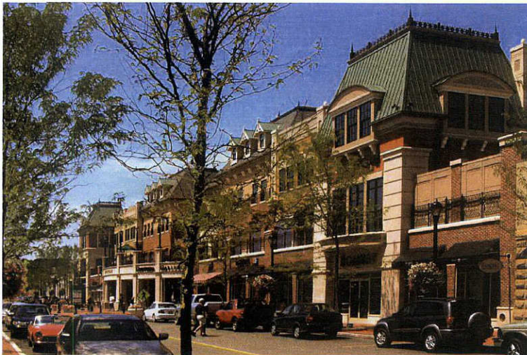
FIGURE 2 On-street parking provides a buffer between pedestrians and vehicles, slows traffic flow, and improves access to services
