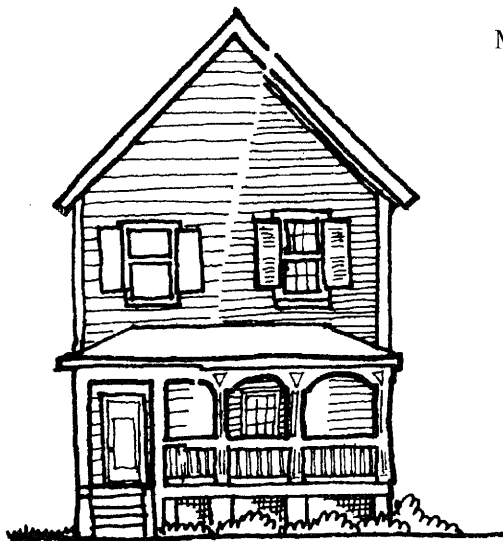
SUBSTITUTE SIDING COVERS ORIGINAL DETAILS
