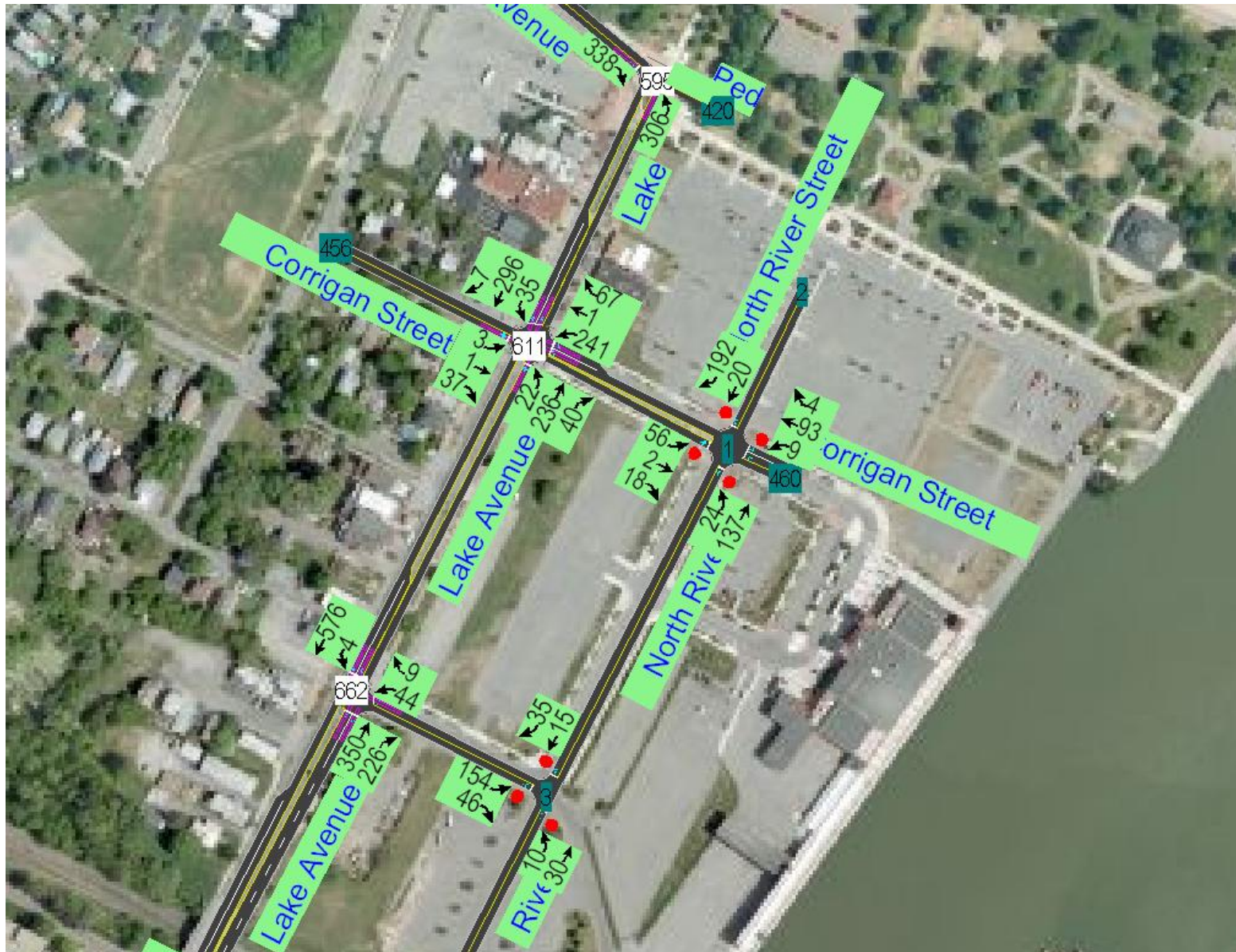
2010 Existing Friday 8:30 – 9:30 PM Peak Hour Intersection Turning Movement Volumes With North River Street Connection between Corrigan Street and Portside Drive
