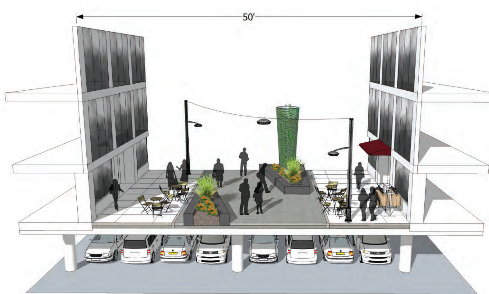
Pedestrian Street typical section
