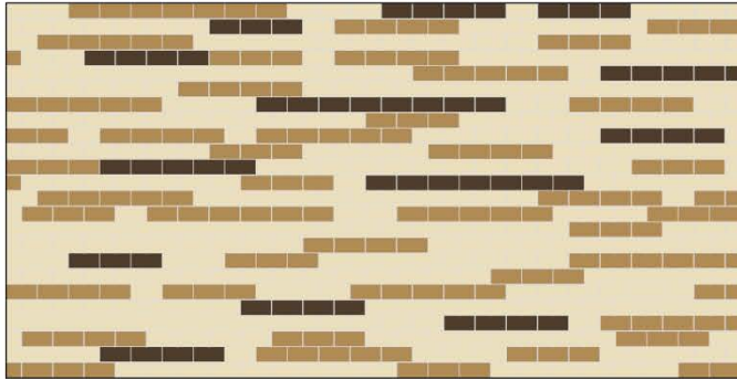
Primary Plaza Surfacing, Hanover Unit Pavers, 3 color blend
