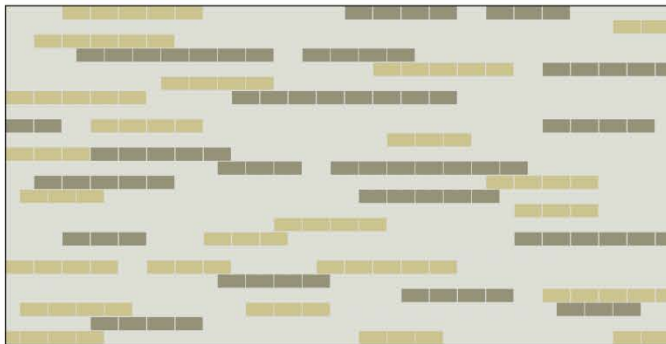
Secondary Plaza Surfacing, Hanover Unit Pavers, 3 color blend
