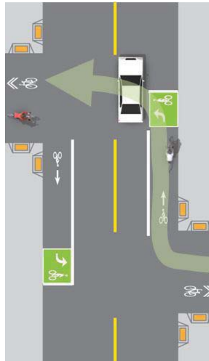
Two Stage Turn Boxes also provide designated spaces for bicyclists to make a crossing in two stages. This treatment should be implemented with signage to show bicyclists & motorists how the treatment works.
