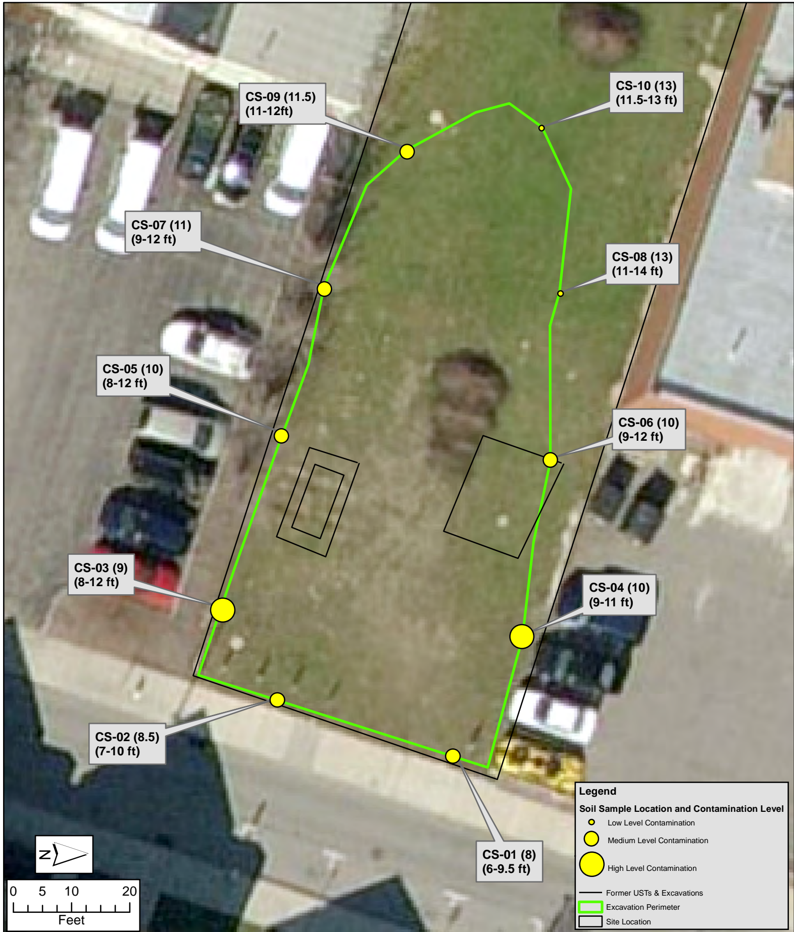
FIGURE 3 CONFIRMATORY SAMPLE LOCATION & CONTAMINANT LEVEL MAP
