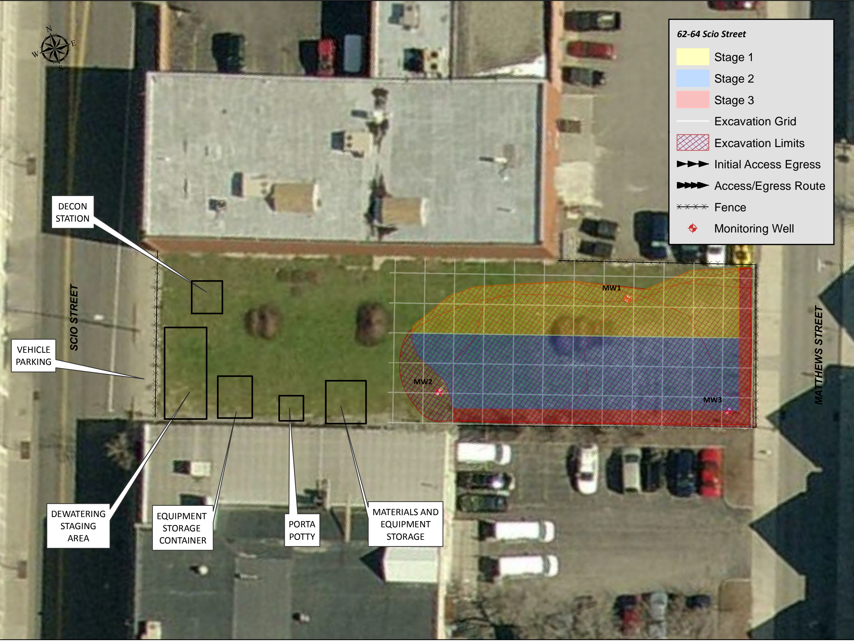
FIGURE 2 IRM LAYOUT AND EXCAVATION SEQUENCING
